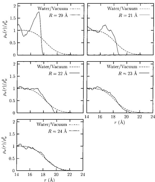
**Figure 4.** water density profile obtained using the repulsive water–wall interaction potential  $u^{\text{rep}}(r;R)$  (eq 6) and  $N = 905$  as a function of the distance from the center of the cavity. See the caption of Figure 3 for other definitions.
