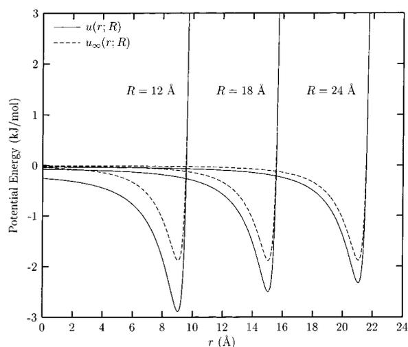
**Figure 2.** Water–hydrocarbon medium interaction potentials  $u(r;R)$  (eq 4) and  $u_\infty(r;R)$  (eq 5) as a function of the radial distance from the center of the cavity of the oxygen atom of a water molecule. The potentials are given for  $R = 12, 18,$  and  $24 \text{ \AA}$  and for  $\rho = 0.0233 \text{ \AA}^{-3}$ .
