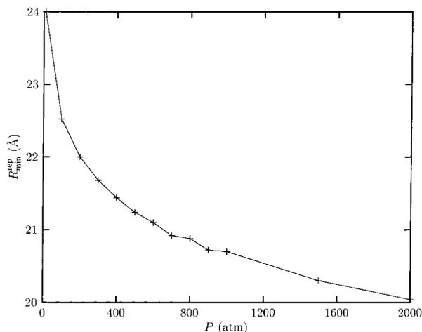
**Figure 6.** Cavity radius at the minimum of the Helmholtz free energy (or, equivalently, of the Gibbs free energy) as a function of applied pressure for the repulsive water–wall interaction  $u^{\text{rep}}(r;R)$ ,  $N = 905$ , and  $\rho = 0.0233$  Å $^{-3}$ .
