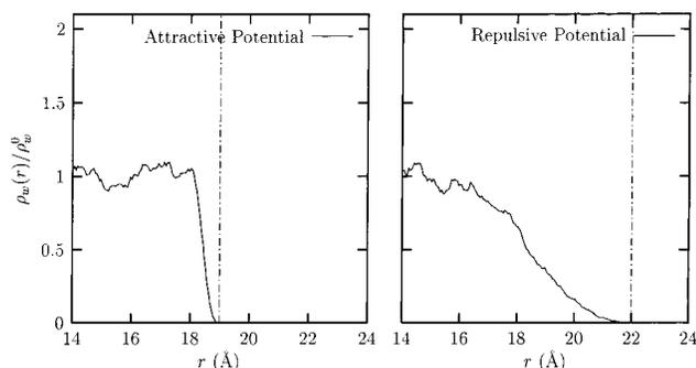
**Figure 7.** Water density profiles of the equilibrium states obtained using the attractive ( $R = 21 \text{ \AA}$ ) and repulsive ( $R = 24 \text{ \AA}$ ) water–wall interaction potential at 10 atm pressure and 298 K. The dash–dotted vertical lines indicate the approximate distance of closest approach between the water molecules and the wall.
