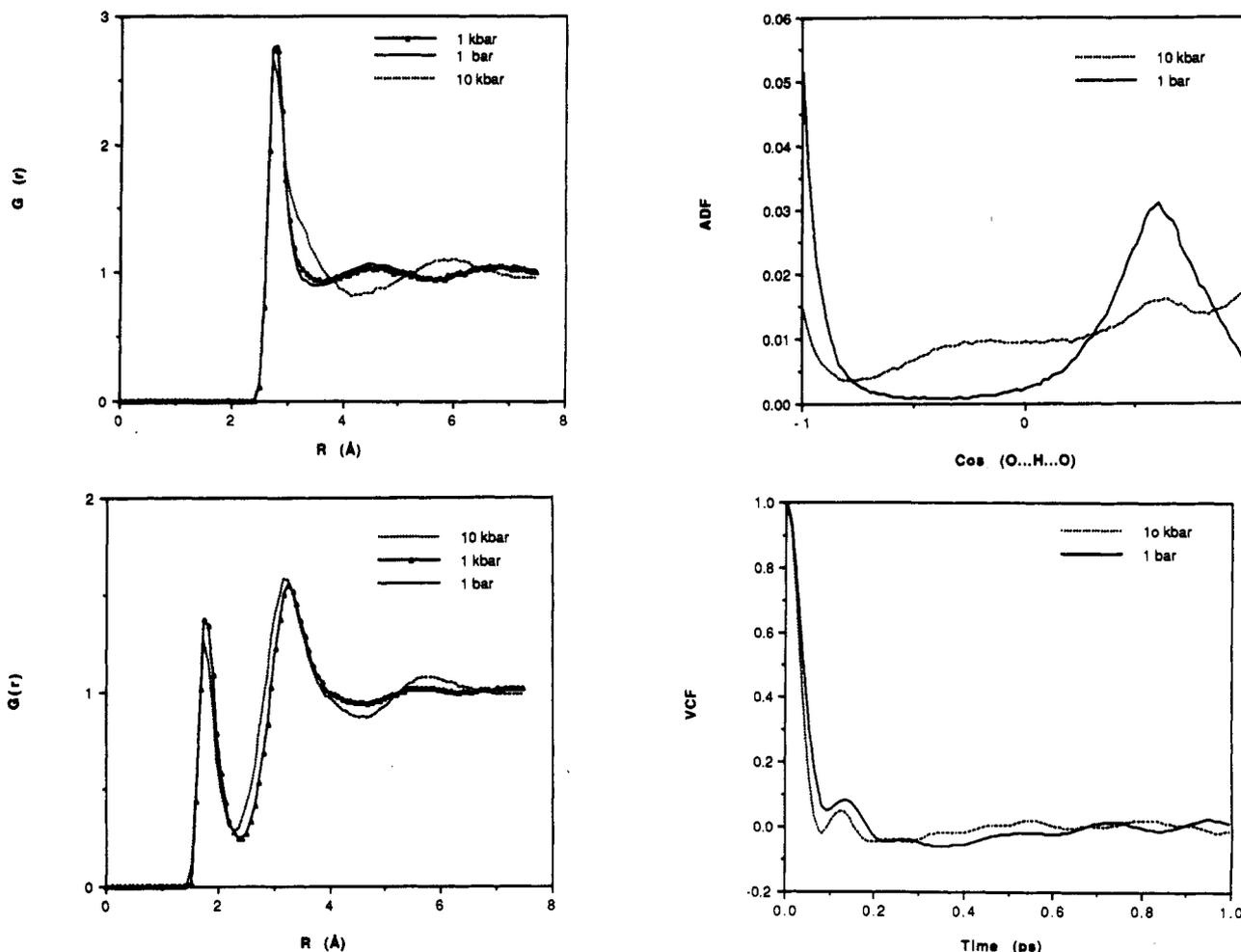
**Figure 1.** Water-water correlation functions: (a, upper left) oxygen-oxygen radial distribution function at 1 bar, 1 kbar, and 10 kbar; (b, lower left) oxygen-hydrogen radial distribution function at 1 bar, 1 kbar, and 10 kbar; (c, upper right) oxygen-hydrogen-oxygen angular distribution function for nearest-neighbor water molecules at 1 bar and 10 kbar; (d, lower right) center of mass velocity correlations function 1 bar and 10 kbar.
