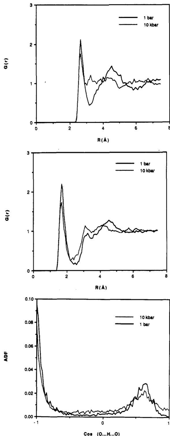
**Figure 2.** Solute-solvent correlation functions from trajectories with ground-state formaldehyde: (a, top) oxygen-oxygen (formaldehyde-water) radial distribution function at 1 bar and 10 kbar; (b, middle) oxygen-hydrogen (formaldehyde-water) radial distribution function 1 bar and 10 kbar; (c, bottom) oxygen-hydrogen-oxygen (formaldehyde-water-water) at 1 bar and 10 kbar.
