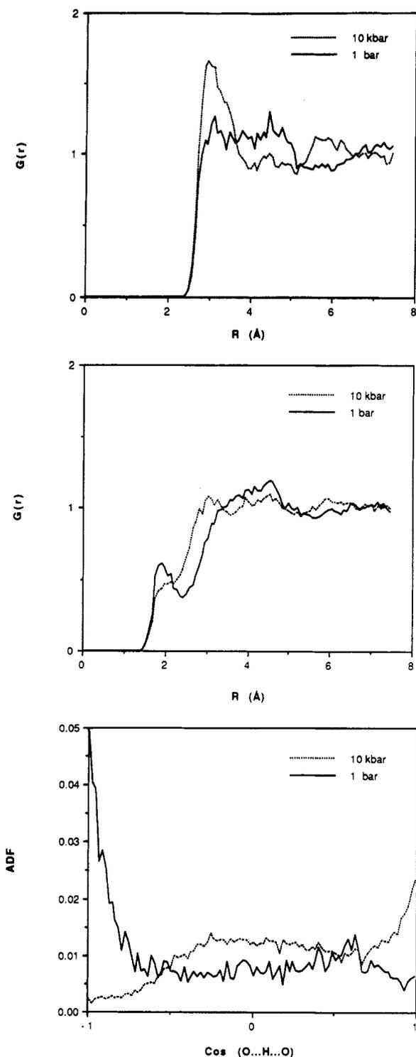
**Figure 3.** Solute-solvent correlation functions from trajectories with excited state formaldehyde: (a, top) oxygen-oxygen (formaldehyde-water) radial distribution function at 1 bar and 10 kbar; (b, middle) oxygen-hydrogen (formaldehyde-water) radial distribution function at 1 bar and 10 kbar; (c, bottom) oxygen-hydrogen-oxygen (formaldehyde-water-water) at 1 bar and 10 kbar.
